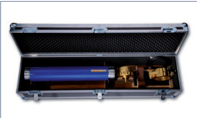
Figure 7b: Test set-up CoMeT 90, supply schedule, box 2
