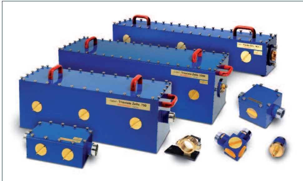
Figure 11: Different designs of Triaxial Cells of the CoMeT System
